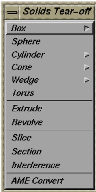
Solid objects can be created from a set of primitives (box, sphere, cylinder, cone, wedge and torus) or sweeping two dimensional elements (extrude, revolve). Extrude works also with closed plines, which can be extruded along complex paths. There is another sort of solid primitives called REGIONS (in menu CONSTRUCT), which are basically two-dimensional solids. A REGION is created after an existing two-dimensional entity, for example, a closed polyline.
